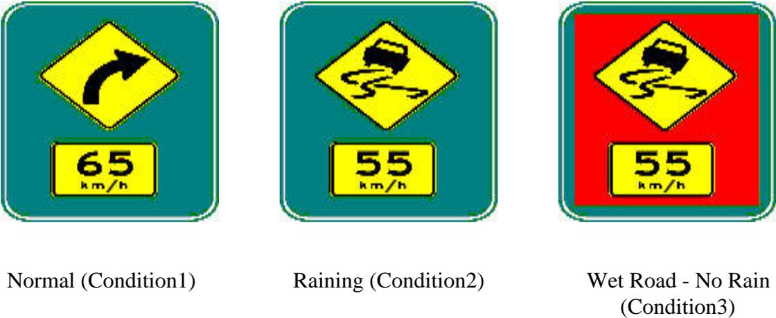
FIG 2: Variable Sign Arrangement
