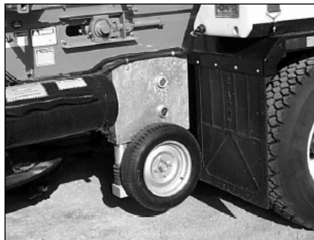
Friction Meter Mounted on Snowplow
