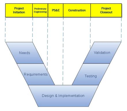
Dashed lines from the traditional process to the Vee process show how the two processes relate to each other. Generally, Project Initiation through Project Closeout is related to the Vee Needs through Validation processes. There is not quite a one-to-one relationship between the different stages or phases of the models, but since each are versions of sequential models, they line up fairly well.
