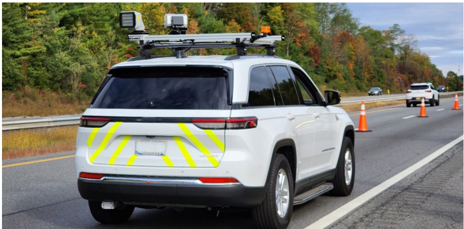
Figure 3. Photo. New York State work zone speed safety camera enforcement vehicle (Source: New York State Department of Transportation (NYSDOT)).
