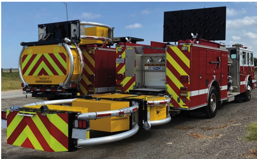
Figure 2. Photo. Surplus fire apparatuses repurposed as blocking vehicles. (Photo Credit: Grand Prairie, Texas, Fire Department.)
