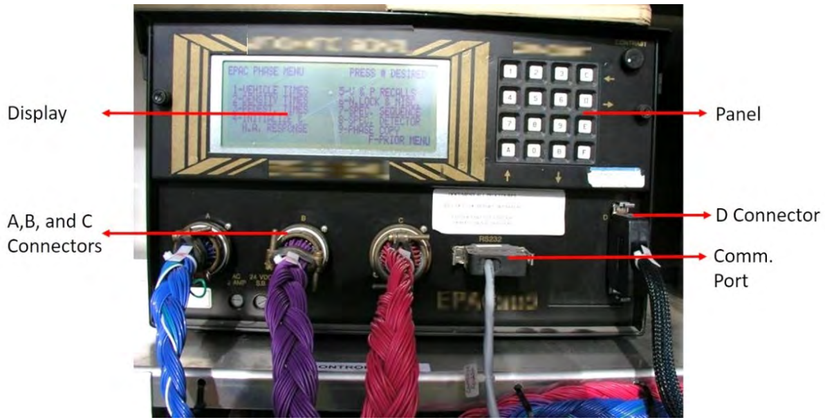
Figure 23. Photograph. Example of a TS1 controller.
