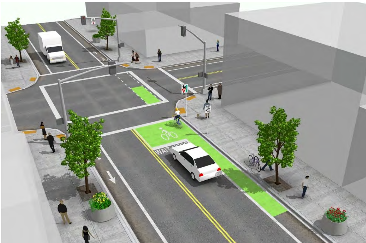
Figure 46. Graphic. Illustration of a bicycle box used at an intersection. (6)
