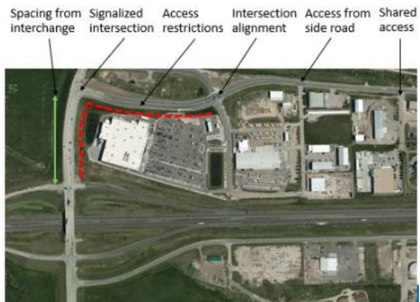
Figure 3.19. Access spacing at a major interchange.
