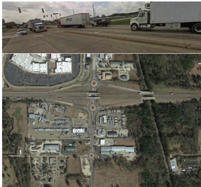
Figure 3.20. Replacement of closely spaced signalized intersections with roundabouts in Louisiana.
