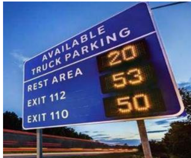
Figure 3.8. Example dynamic parking capacity sign.
