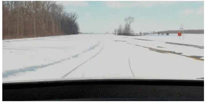
Figure 6. Winter Field Test #2 Vehicle A following the piled up snow in the travel lane and deviating to the adjacent lane. Source: FHWA
