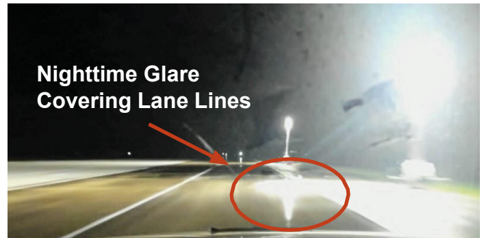
Figure 3. Nighttime glare conditions covering lane lines and creating perception challenges for test vehicles during Summer Field Test #1. Source: FHWA
