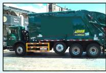
Steel or Aluminum Rail Side Guard On rail-style side guards, continuous horizontal rails provide a smooth impact surface, while the spaces between rails enable access to hydraulic levers, etc. Rail-style guards were custom built for Boston, but they could be made as a configurable, off-the-shelf system, similar to the predominant side guards used on European and Asian trucks.
