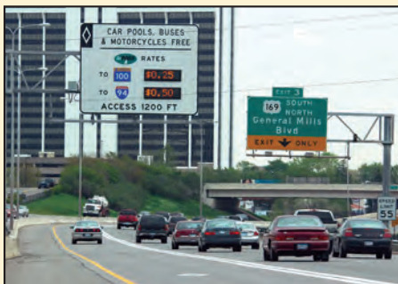
Minnesota DOT Dynamically Priced High Occupancy Toll (HOT) Lanes – Source: U.S. DOT
