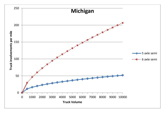
Figure 2: Truck Involvements per Mile versus Truck Volume for Six-Axle Alternative Truck Configurations and Five-Axle Configurations in Michigan
