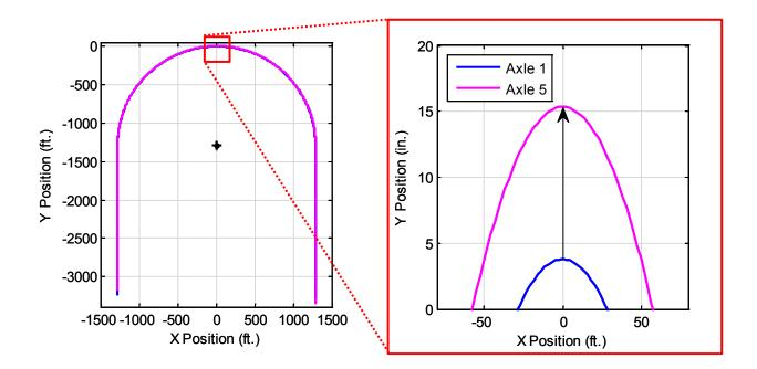
Figure C4. High-speed Off-tracking Path Differences
