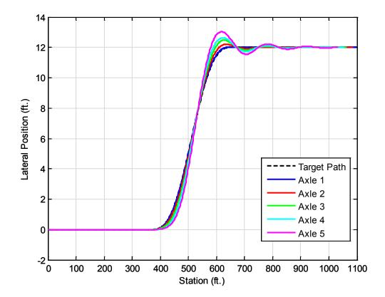
Figure 13: Paths of the Axle centerlines of the Control Double as it Executes the 12-ft.
