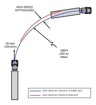
Figure 8: Trailer Tracks to the Outside of the Curve Centerline in this High-Speed Offtracking Illustration.
