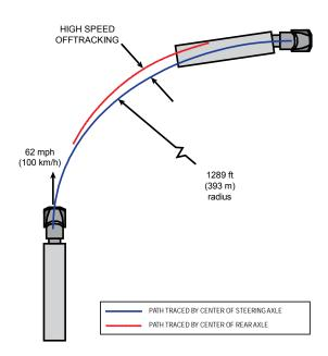
Figure C3. The Simulated High-speed Off-tracking Maneuver.
