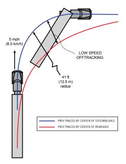
Figure 6: Low-Speed Off-tracking Maneuver Simulates an Intersection
