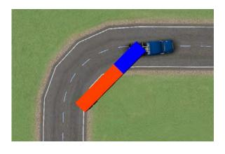
Figure 7: Off-tracking of the Drive and Trailer Axles Rises and Falls During the Maneuver.
