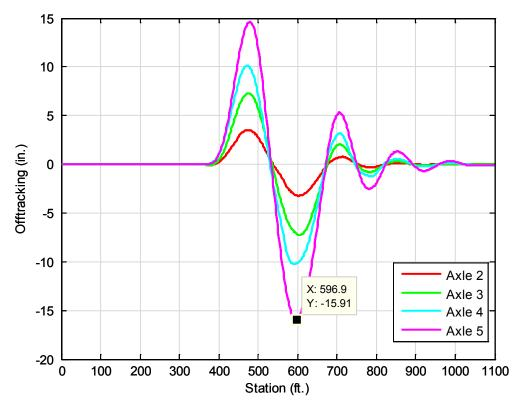
Figure 14: Off-tracking was Computed from the Axle Paths in the Previous Figure<sup>3</sup>
