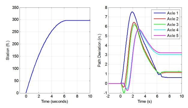
Figure 11: Position vs. Time (left) and Path Deviation vs. Time (right) of Control Single Vehicle as it Stops with Brake Failure on the Right Ends of the Two Drive Axles
