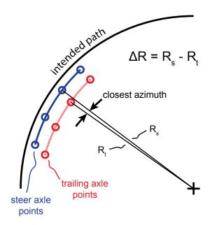
Figure C2. The Low-speed Off-tracking Calculation Points.
