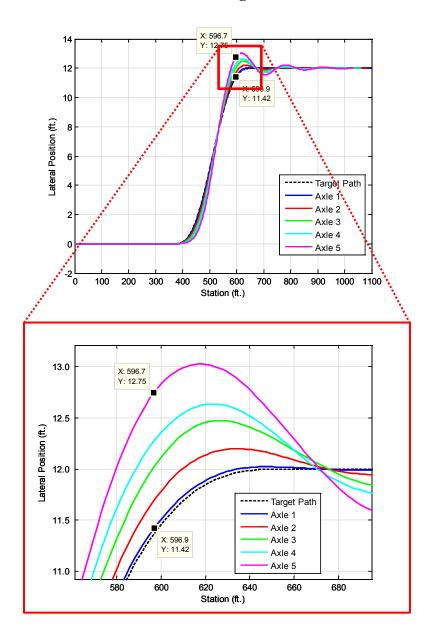
Figure C-7. Maximum Off-tracking for All Excitation Frequencies
