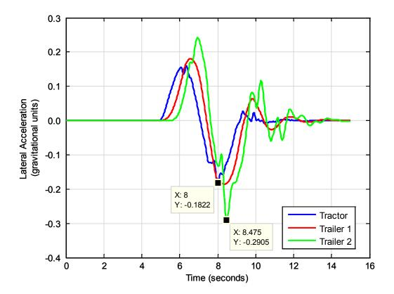
Figure 15: Lateral Acceleration Time Histories of the Three Units of Control Vehicle CD in the 12-ft Lane Change.<sup>4</sup>
