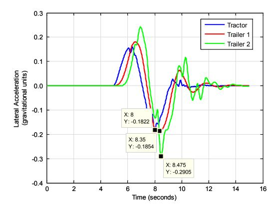
Figure C8. Rearward Amplification Reflected by Peak Lateral Acceleration in Trailers
