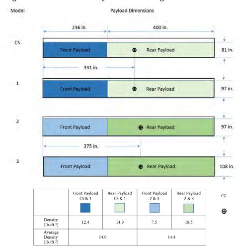
Figure D1. Dimensions of Payloads on the Single-Trailer Combinations
