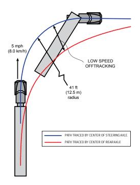
Figure C-1. The Low-speed Off-tracking Maneuver.
