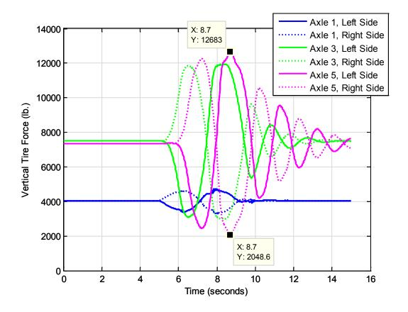
Figure 16: Vertical Tire Forces during the Lane Change Maneuver for the 12-ft Lane Change for Control Vehicle CD<sup>5</sup>
