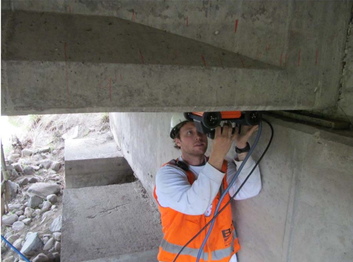
Figure 2 showing GPR scan along bottom of a girder (typical).
