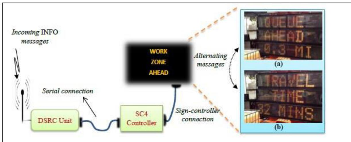
Schematic of DSRC-enabled VMS deployment which allows non-DSRC vehicles to benefit from the technology (University of MN<sup>1</sup>)
