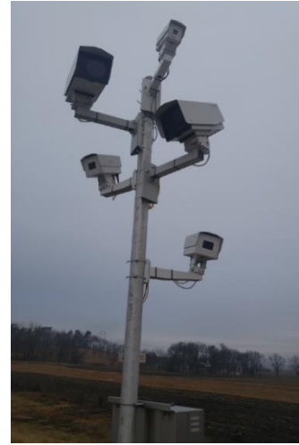
Figure 6 – Example Assembly with License Plate Reader, USDOT Number Reader, and Overview Camera (Jasper County, IA)
