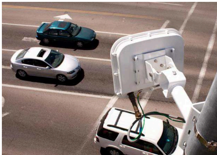
Figure 7. Radar unit being tested by ACHD
