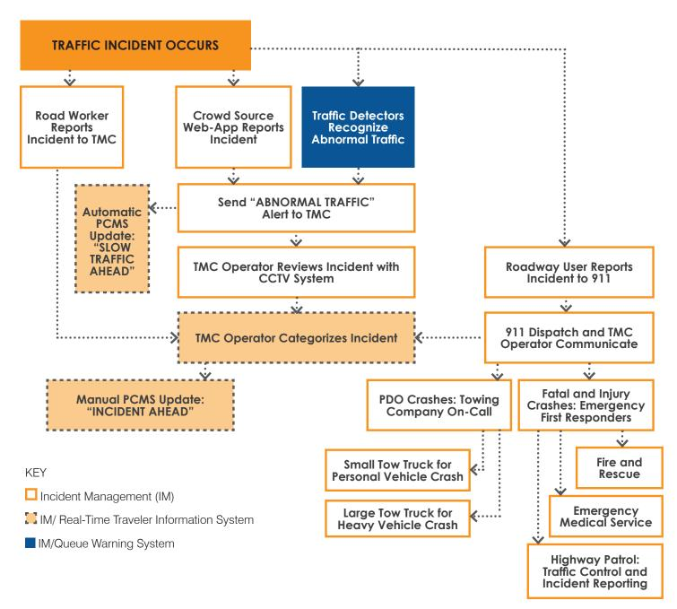
Figure 9. Diagram. Incident management diagram. Source: FHWA.
