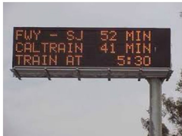
Figure 27. Photo. Variable message sign comparing driving the route with parking and taking transit. (53) (Source: California Department of Transportation).
