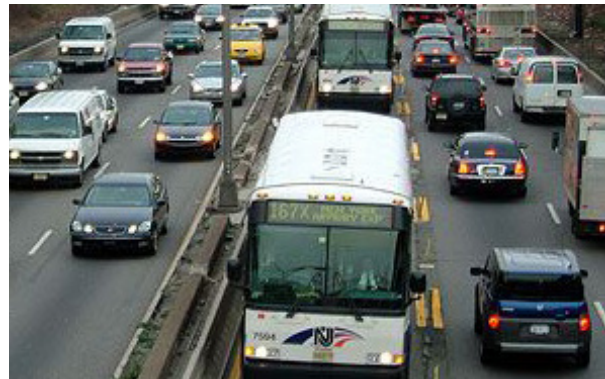
Figure 24. Photo. Buses traveling in the exclusive bus lane. (50) (Source: Port Authority of New York and New Jersey).
