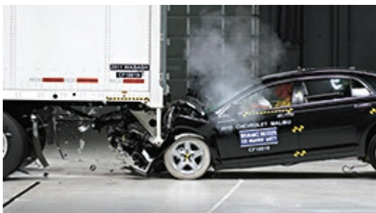
Figure 4. Photo. Stronger under-ride guards, as shown in this photo, reduce deaths and injuries in rear-impact crashes.
