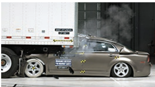
Figure 3. Photo. Inadequate under-ride guards contribute to deaths and injuries in rear-impact crashes, as shown here.
