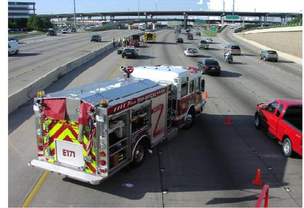
Accordingly, traffic control device placement is also determined by the expected duration of the incident. Upon arrival, responders should estimate the expected duration for recovery using the *MUTCD* guidelines (Minor – under 30 minutes; Intermediate – from 30 minutes to 2 hours; Major – over 2 hours).
