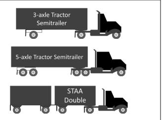
Longer Combination Vehicles –A subgroup of combination trucks, LCVs are double and triple trailer combinations that can exceed 80,000 lbs. on Interstate Highways in 23 States. All vehicles have seven or more axles consisting of three or more units, one of which is a tractor or a straight truck power unit. Three common LCVs are in operation across the U.S:
