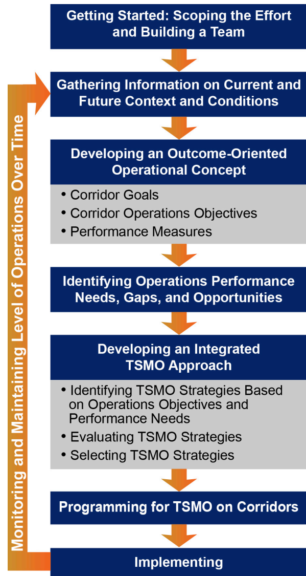
Figure 8. Diagram. Approach to planning for transportation systems management and operations within corridors.
