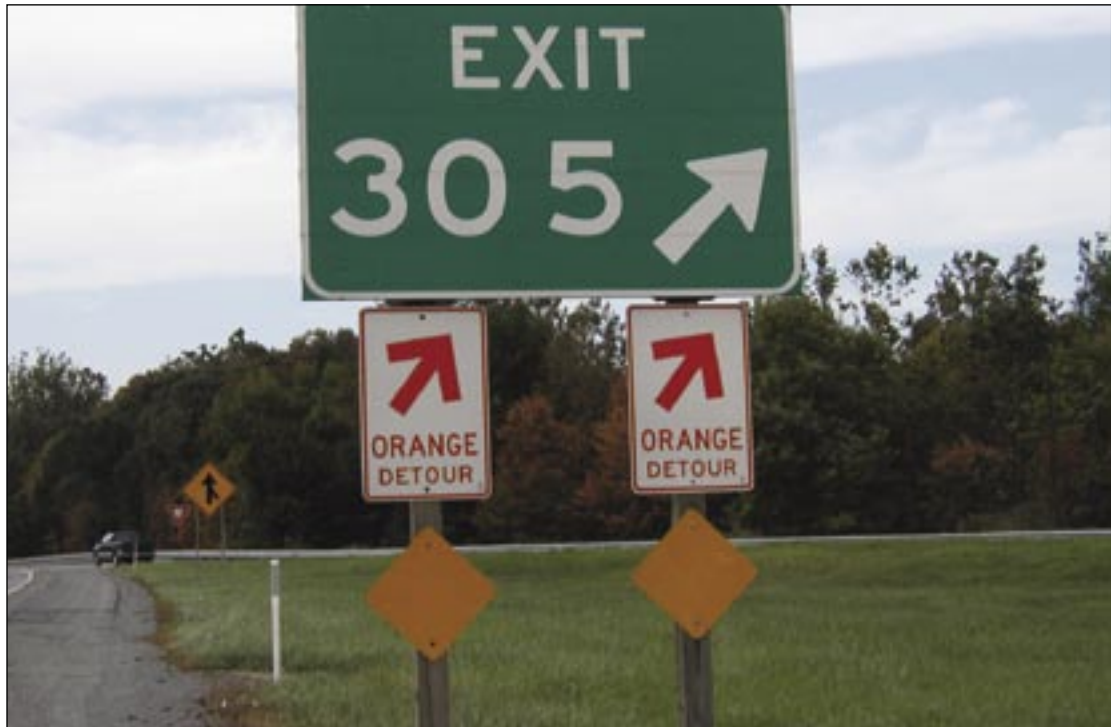
Figure 6-1. Color-coded alternate route trailblazer sign.
