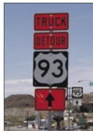
Figure 2-7. Truck detour route trailblazer.
