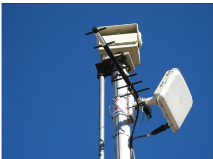
Figure 3-5. Delays can be Estimated from a Series of Spot Speed Sensors along the Roadway Segment
