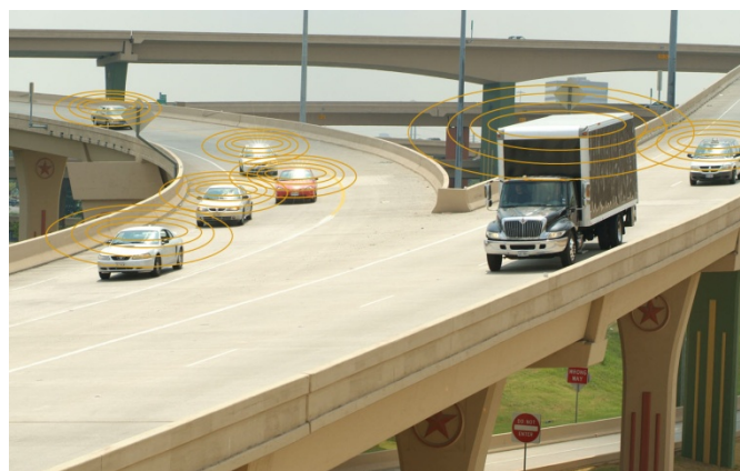
Figure 3-4. The Connected Vehicle Initiative involves Communication between Vehicles and between Vehicles and Roadside Infrastructure
