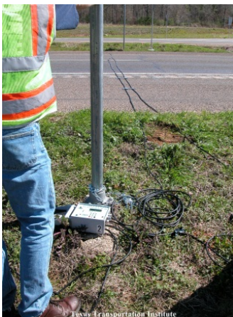
Figure 3-3. Mechanical Counters can Sample Throughput and/or Demand Volumes at a Work Zone
