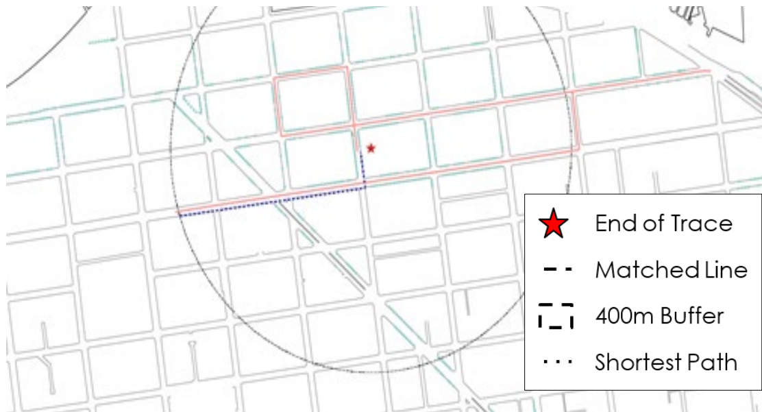
Figure 5. Illustration. Cruising: identified when paths traveled exceed shortest paths.
