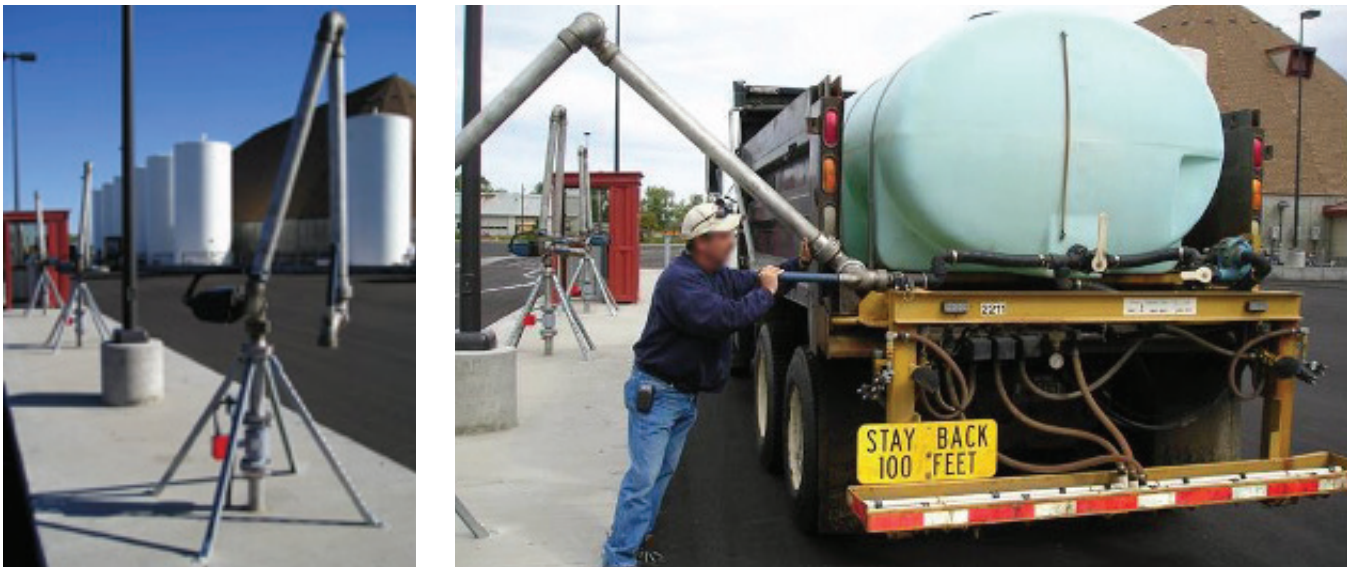
Figure 4. Spring-loaded arms (left) can quick-attach to snowplows (right) for fast loading of liquid deicing material. (Source: City of Fort Collins).
