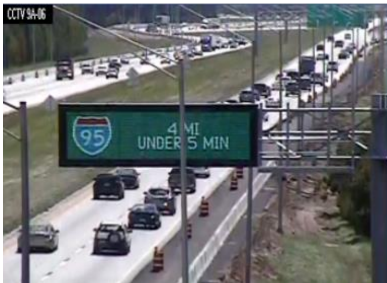
Figure 1. Photo. Route shield on a full-matrix color changeable message sign (CMS). Source: Florida Department of Transportation
