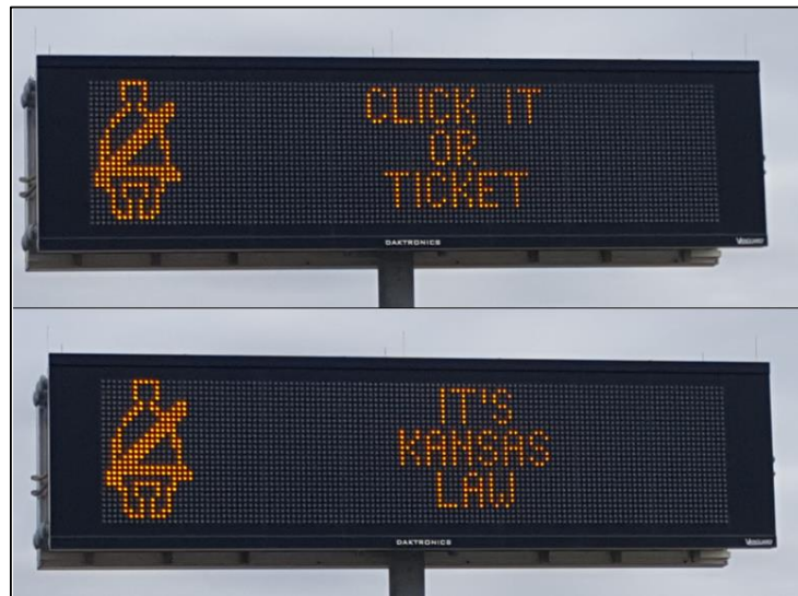
Figure 2. Photo. An example of a multi-phase message displayed on a changeable message sign (CMS).
