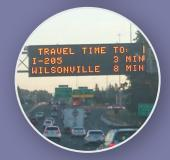
The Wilmington Area Planning Council's CMP has identified a strategy evaluation process that prioritizes improving roadway operations above adding capacity. To that end, the region has increased its investment in technologies for monitoring traffic conditions with speed detectors and traffic cameras and communicating to the traveling public using variable message signs.
