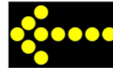
Figure 8. Arrow Panel Indicating a Blocked Lane.
