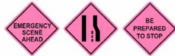
Figure 12. Incident Advance Warning Signs.
